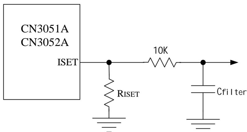
Figure 5 Isolating Capacitive Load on ISET Pin
