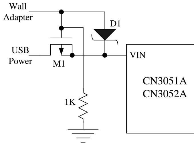
Figure 4 Combining Wall Adapter and USB Power
