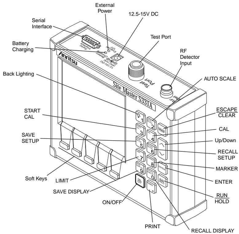
Figure 2-1. *Site Master Controls and Connectors*
