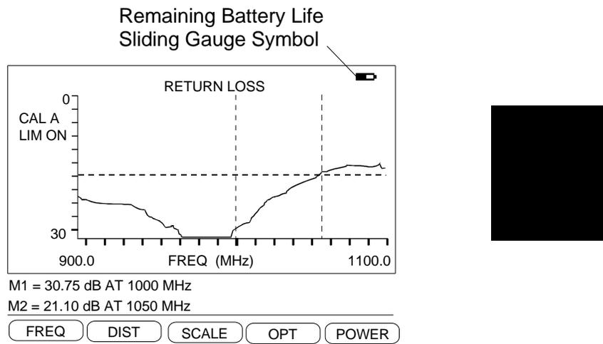
Figure 2-8. Battery Monitor
