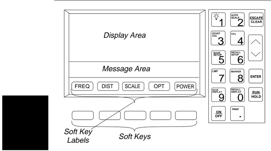
Figure 2-2. Site Master Front Panel Display Layout
