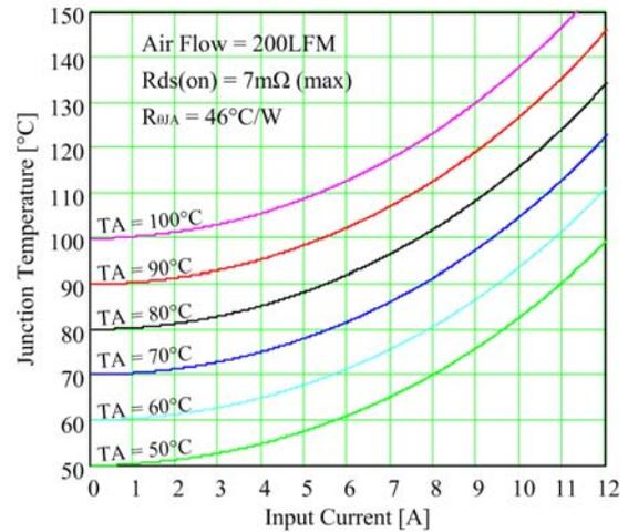
**Figure 14:** Junction Temperature vs. Input Current (200LFM)
