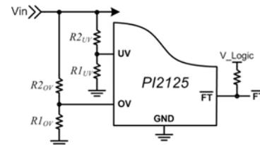
Figure 21: UV & OV two-resistor divider configuration
