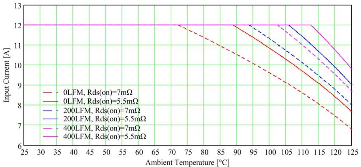
**Figure 17:** PI2125 input current de-rating based on maximum T<sub>J</sub>=150°C vs. ambient temperature
