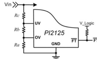
Figure 20: UV & OV three-resistor divider configuration
