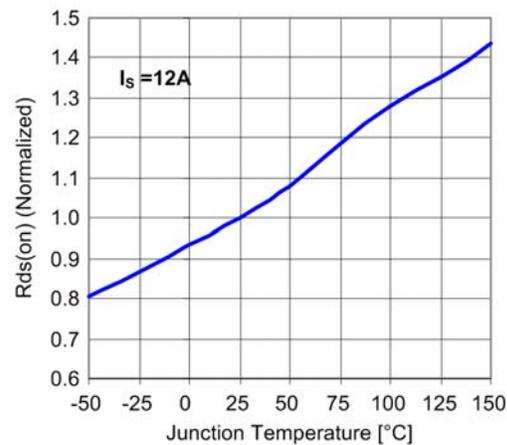
**Figure 11:** Internal MOSFET on-state resistance vs. temperature
