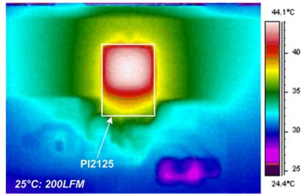
**Figure 16:** PI2125 mounted on PI2125-EVAL
