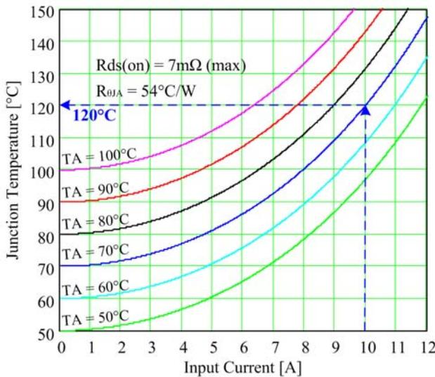
**Figure 22:** Example 1 final junction temperature at 10A/70°C  $T_A$
