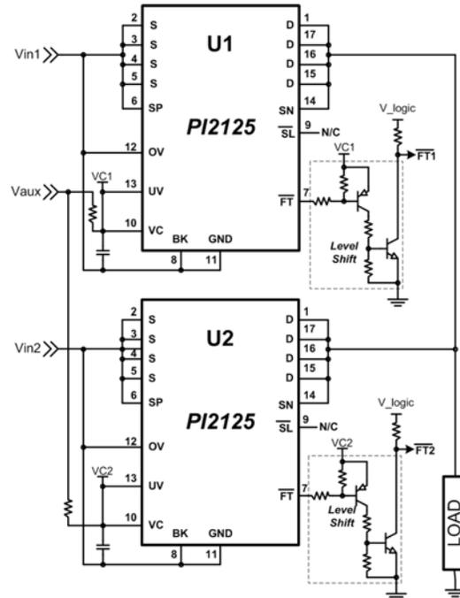
**Figure 23:** PI2125, 12V floating Active ORing application
