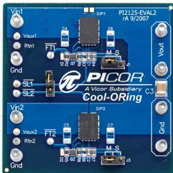
Figure 25: PI2125 Mounted on PI2125-EVAL2
