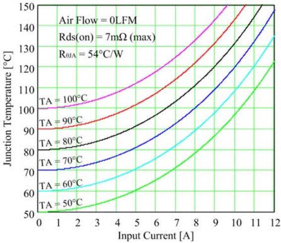
**Figure 13:** Junction Temperature vs. Input Current (0LFM)
